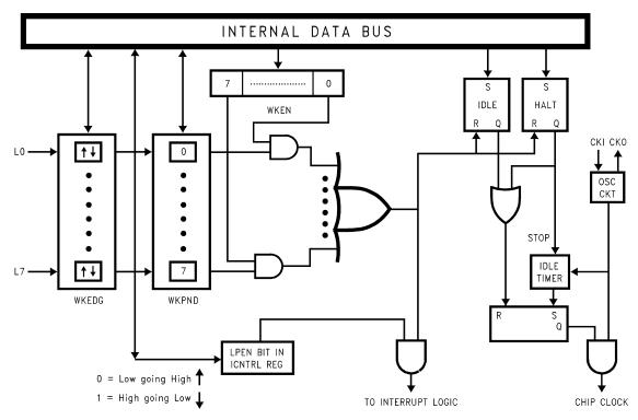
Figure 29. Multi-Input Wake Up Logic
