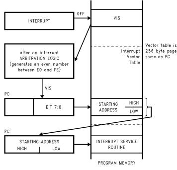
Figure 35. VIS Operation
