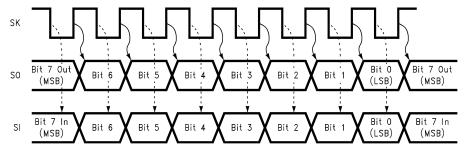
Figure 40. MICROWIRE/PLUS SPI Mode Interface Timing, Normal SK Mode, SK Idle Phase being High
