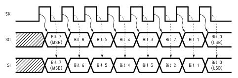
Figure 39. MICROWIRE/PLUS SPI Mode Interface Timing, Alternate SK Mode, SK Idle Phase being Low
