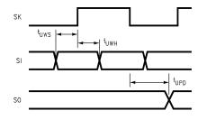
Figure 8. MICROWIRE/PLUS Timing
