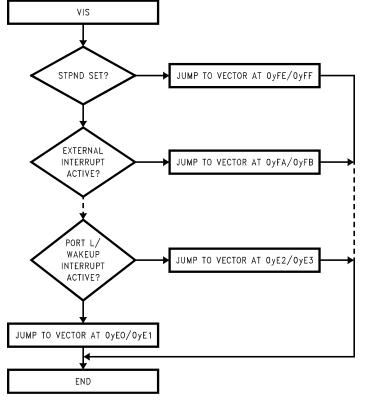
Figure 36. VIS Flowchart
