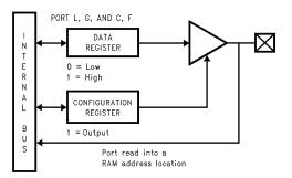
Figure 14. I/O Port Configurations—Output Mode
