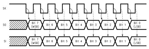
Figure 41. MICROWIRE/PLUS SPI Mode Interface Timing, Alternate SK Mode, SK Idle Phase being High
