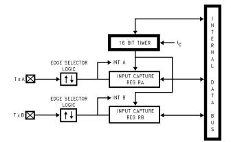
Figure 26. Timer in Input Capture Mode
