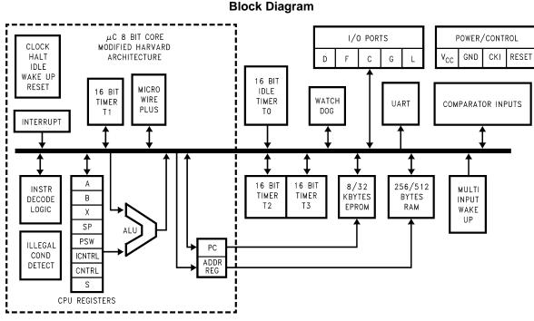
Figure 1. COP8SGx Block Diagram
