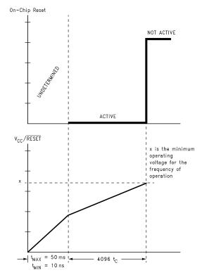
Figure 19. Reset Timing (Power-On Reset Enabled) with V<sub>CC</sub> Tied to RESET
